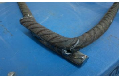
Crack/bond failure in bend test
