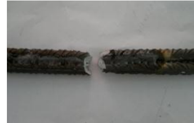
Failure of a specimen in G3
