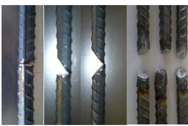
Prepared/failure bars in G6
