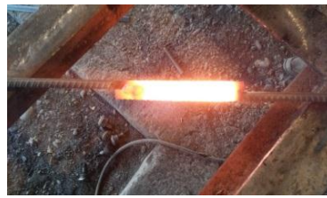
Heat input during welding
