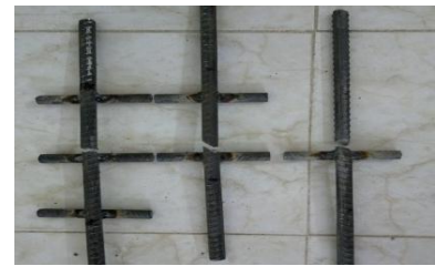
Failure planes for G4
