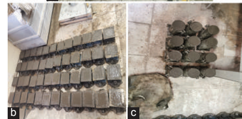
Fig. 2. (a) Trial mix, (b) cube sample for compressive strength, and (c) cylinder sample for splitting tensile strength.
