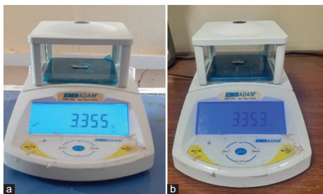
Fig. 7. (a) Coupon on the weight scale before use. (b) Coupon on the weight scale after use.
