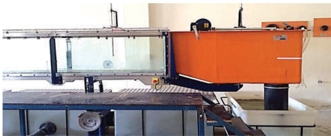
Fig. 3. Location of the overshot gate in the laboratory flume.
