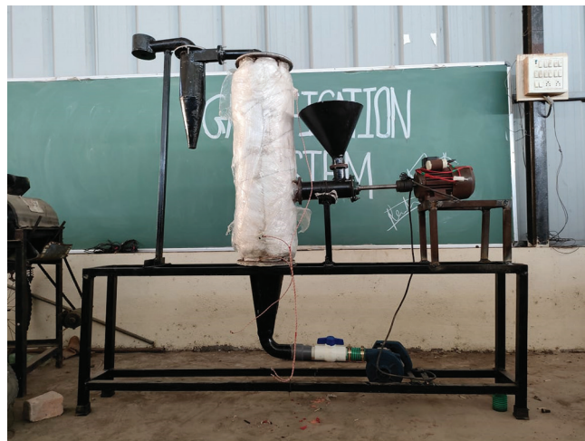
Fig. 3. Bubbling fluidized bed Gasifier setup.
