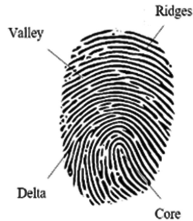
Fig. 2. Fundamental structural features in fingerprint biometrics.
