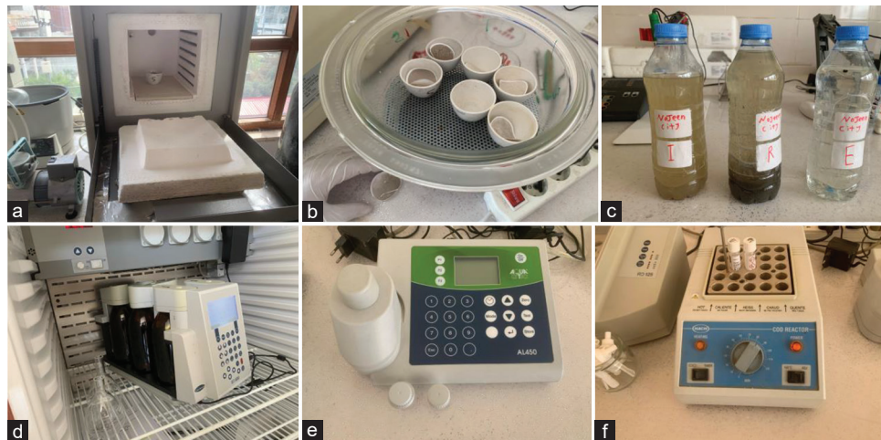
Fig. 3. Wastewater samples and laboratory instruments used in this study. (a) Collected samples, (b) Desiccator, (c) volatile suspended solids furnace, (d) chemical oxygen demand digester, (e) Multi-test Photometer, (f) biochemical oxygen demand respirometric system.
