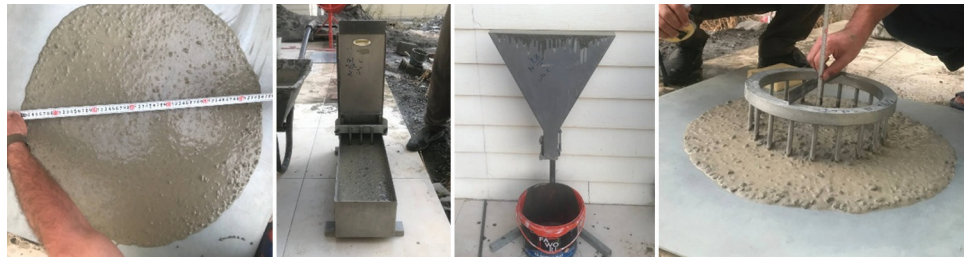
Fig. 2. Self-compacting concrete fresh tests.
