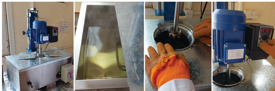
Fig. 1. Mixing procedure to produce nanosilica-modified asphalt cement.
