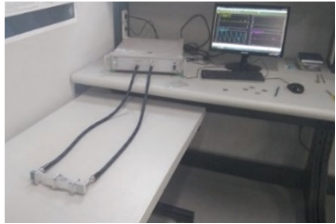
Fig. 8. Measurement set-up for the combined fractal structure 2 \times 2 -unit cell with dimensions of 22.86 \text{ mm} \times 22.86 \text{ mm} .
