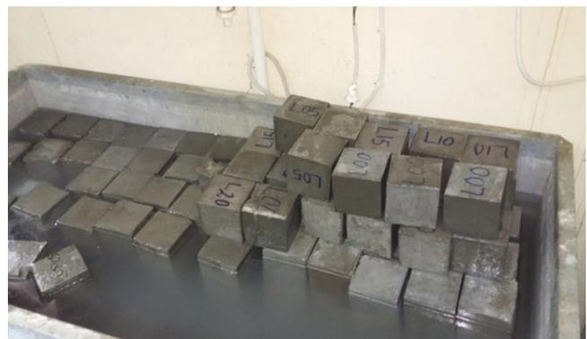
Fig. 2. Some of cubes and prisms during curing.
