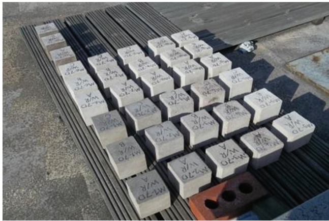
Fig. 2. Outside weathering exposure
