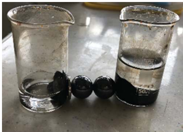
Fig. 2. Magnetite nanoparticles separated by using an external magnetic field.
