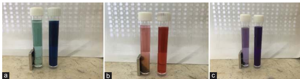
Fig. 10. Magnetite nanoparticles applied of Dyes (a) malachite green, (b) safranin and (c) chrystal violet.
