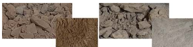
Fig. 1. Alum sludge waste materials. (a) Alum sludge oven-dried at 110°C. (b) Alum sludge furnace-burned at 700°C.
