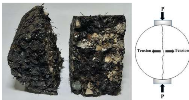
Fig. 16. Failure mode of indirect tensile test.
